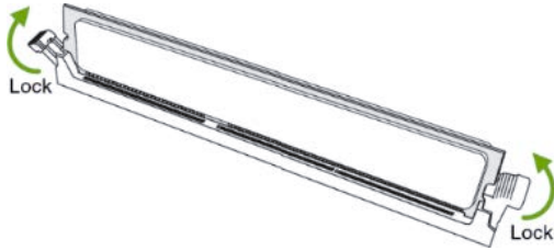
Figure 26. Locking a new memory module into its slot
