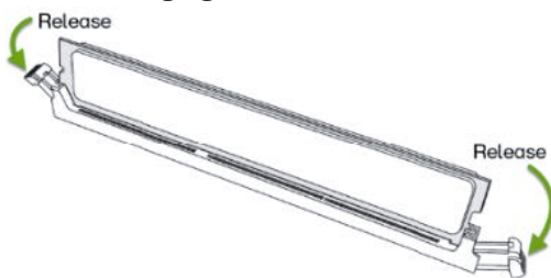
Figure 23. Releasing a memory module from its slot
